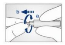
1.Carefully twist off the protective cap until it is separated from the device.
